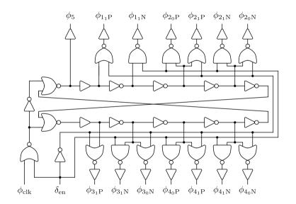
▲ (4+1)-phase switching scheme to avoid signal-dependent charge injections that would cause distortion [8]
