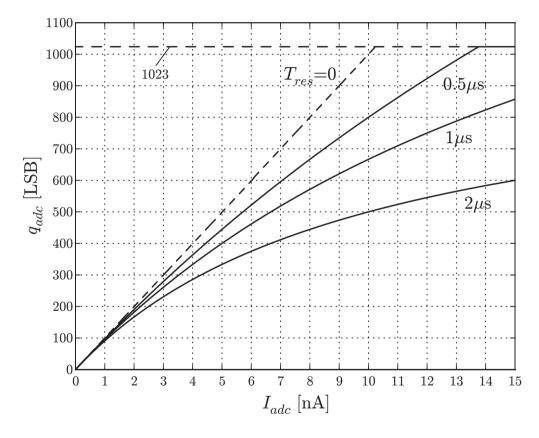
e.g.  $C_{int} = 100 \mathrm{fF}$ ,  $V_{th} = 200 \mathrm{mV}$ ,  $T_{caq} = 2 \mathrm{ms}$  and  $10 \mathrm{bit}$  output
