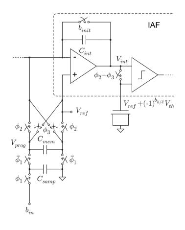
▲ Reuse of ADC CMOS circuit for compact area
