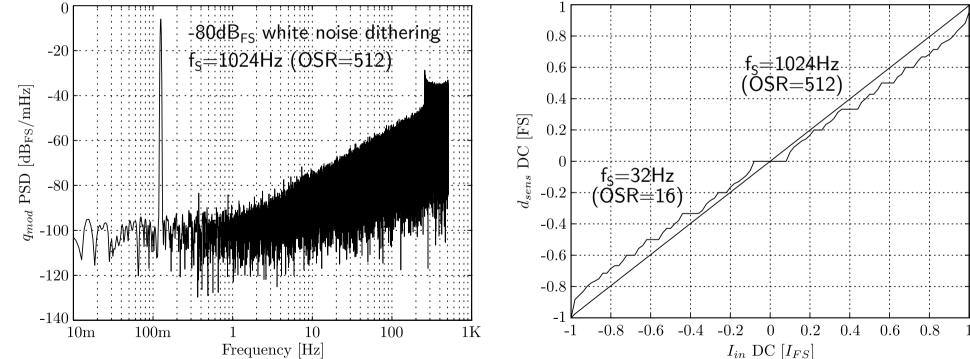
e.g.  $\Delta\Sigma M$  behavioral simulation for  $R_{ctw}=500k\Omega$ ,  $\tau_{ch}=0.16s$ ,  $V_{ref}=1V$  and  $I_{ES}=2\mu A$
