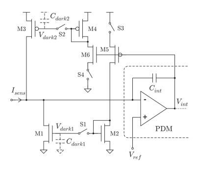
▲ Reuse of ADC CMOS circuit for compact area
