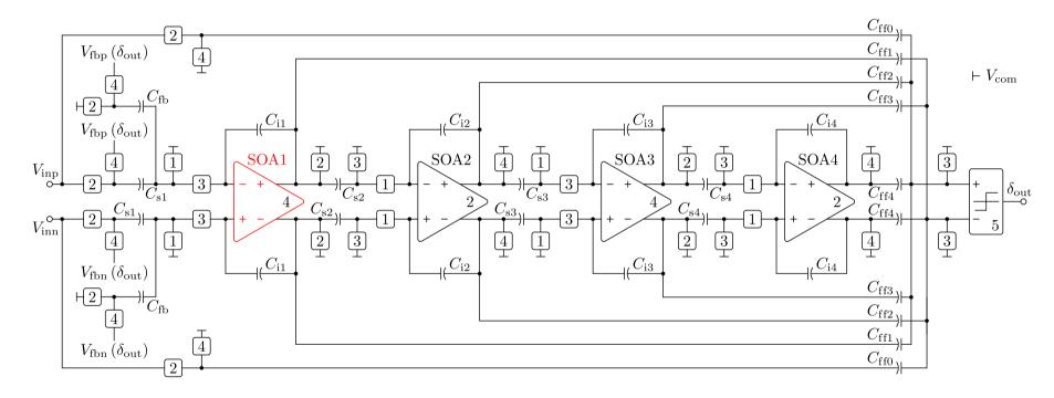
Large capacitor sizing [pF] according to kT/C specs and optimal coefficients [8]:
