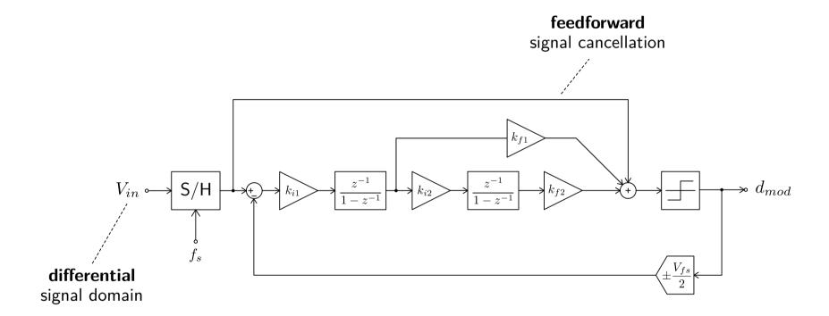
► Fully-differential 2nd-order single-bit DSM example:
