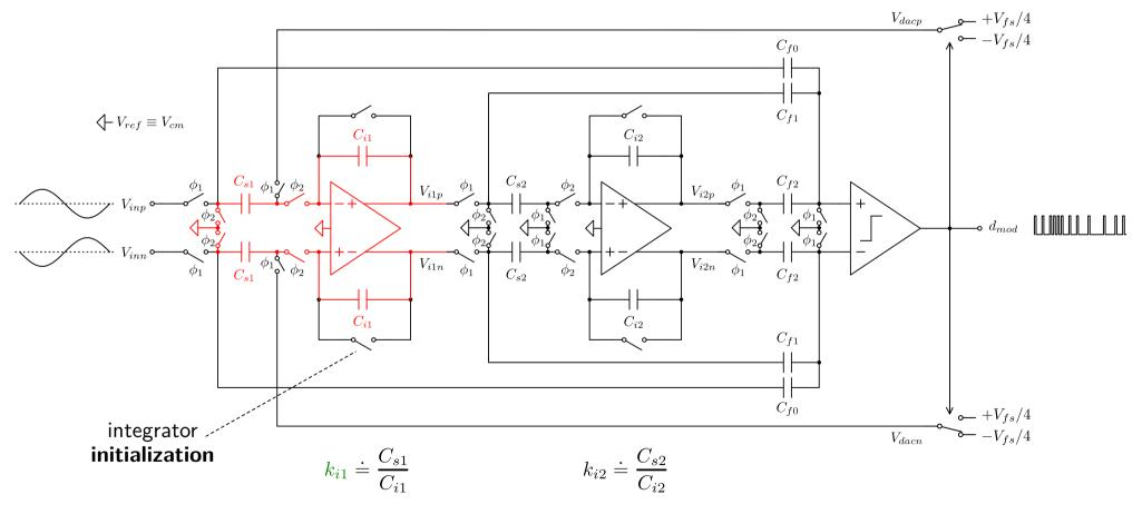
► Fully-differential 2nd-order single-bit DSM example:
