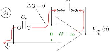
$$V_{out}(n) = V_{out}(n-1) + \frac{C_s}{C_i}V_{in}(n-1)$$
