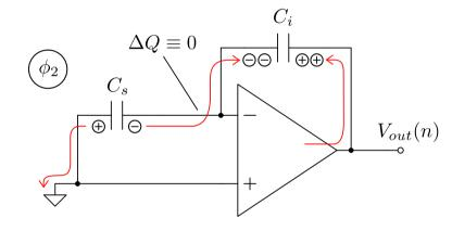
$$V_{out}(n) = V_{out}(n-1) + \frac{C_s}{C_i}V_{in}(n-1)$$
