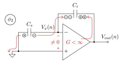
integration **leakage** gain **mismatch**
