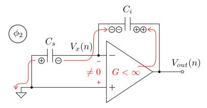
integration **leakage** gain **mismatch**
