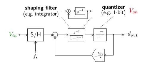
$$D_{out} = STF(z)V_{in} + NTF(z)V_{qn} \begin{cases} STF = \frac{H}{1+H} & \to 1 \\ H \to \infty \\ NTF = \frac{1}{1+H} & \to 0 \end{cases}$$
