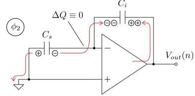
$$V_{out}(n) = V_{out}(n-1) + \frac{C_s}{C_i}V_{in}(n-1)$$
