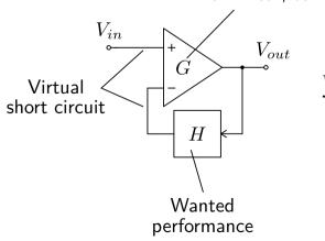
$$\frac{V_{out}}{V_{in}} = \frac{G}{1 + GH} \simeq \frac{1}{H}$$
