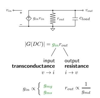
► Enhancement by increasing MOSFET input transconductance?
