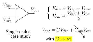
▲ Analog computing **operations** in closed loop:
