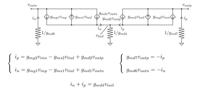
$$\begin{split} (g_{md7} + g_{md2})v_{outp} - (g_{md6} + g_{md1})v_{outn} + \frac{g_{ms1} - g_{ms2}}{g_{ms1} + g_{ms2} + g_{md4}}(g_{md2}v_{outp} + g_{md1}v_{outn}) = \\ & = g_{mg1}v_{inp} - g_{mg2}v_{inn} + \frac{g_{ms2} - g_{ms1}}{g_{ms1} + g_{ms2} + g_{md4}}(g_{mg1}v_{inp} + g_{mg2}v_{inn}) \end{split}$$
