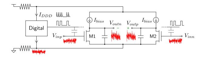
$$\begin{cases} V_{outd} \doteq V_{outp} - V_{outn} \\ V_{outc} \doteq \frac{V_{outp} + V_{outn}}{2} \end{cases}$$
