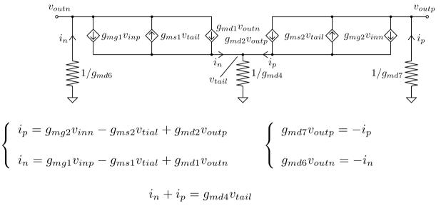
$$\begin{array}{c} \textbf{differential output} \\ v_{outd} \\ (g_{md7} + g_{md2})v_{outp} - (g_{md6} + g_{md1})v_{outn} + \frac{g_{ms1} - g_{ms2}}{g_{ms1} + g_{ms2} + g_{md4}} (g_{md2}v_{outp} + g_{md1}v_{outn}) = \\ \\ = g_{mg1}v_{inp} - g_{mg2}v_{inn} + \frac{g_{ms2} - g_{ms1}}{g_{ms1} + g_{ms2} + g_{md4}} (g_{mg1}v_{inp} + g_{mg2}v_{inn}) \\ \\ v_{ind} \\ \\ \textbf{differential input} \\ \end{array}$$
