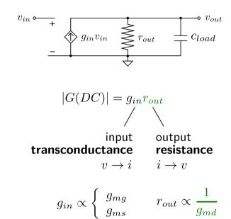
► Enhancement by increasing MOSFET **output impedance**?
