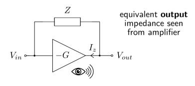
$$Z_{out} \doteq \frac{V_{out}}{-I_z} = \frac{V_{out}}{V_{out} - V_{in}} Z = \frac{G}{1 + G} Z$$
