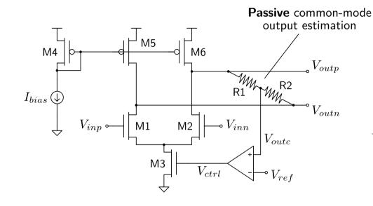
$$V_{outc} = \frac{R_2}{R_1 + R_2} V_{outp} + \frac{R_1}{R_1 + R_2} V_{outn}$$
