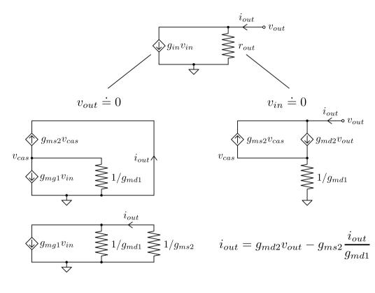
$$g_{in} \doteq \frac{i_{out}}{v_{in}} = g_{mg1} \frac{g_{ms2}}{g_{ms2} + g_{md1}}$$
