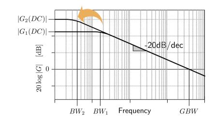
$$BW = \frac{1}{2\pi r_{out} c_{load}} \qquad GBW = \frac{g_{in}}{2\pi c_{load}}$$
