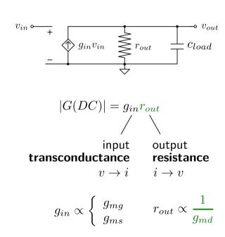
► Enhancement by increasing MOSFET **output impedance**?
