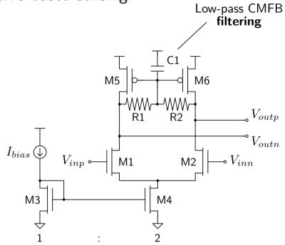
$$V_{outc} = V_{DD} - V_{TH} - \sqrt{\frac{2nI_{bias}}{eta_{5,6}}}$$
