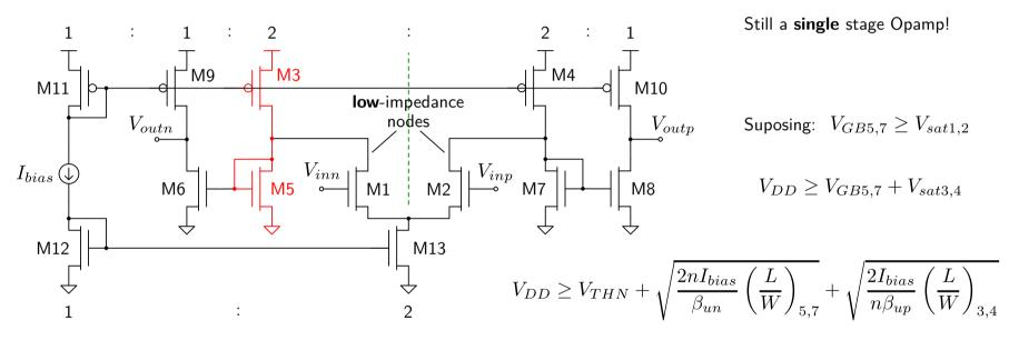
$V_{DDmin} \simeq 1$  threshold + 2 saturation voltages
