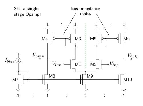
$$V_{sat10} < V_{outp} < V_{DD} - V_{sat6}$$
