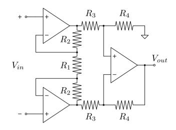
$$\frac{V_{out}}{V_{in}} = \left(1 + \frac{2R_2}{R_1}\right) \frac{R_4}{R_3}$$
