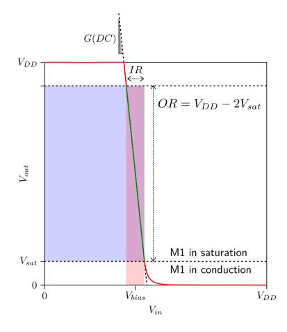
$$V_{sat} = \frac{V_{GB} - V_{TH}}{n} = \frac{V_{bias} - V_{TH}}{n} = \sqrt{\frac{2I_{bias}}{n\beta}}$$
