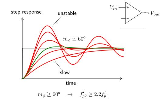
$$f'_{p2} = \frac{g_{mg6}}{2\pi(c_{load} + c_{comp})}$$
