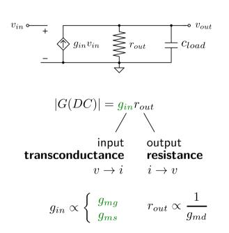
► Enhancement by increasing MOSFET input transconductance?
