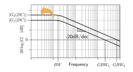
$$BW = \frac{1}{2\pi r_{out} c_{load}} \qquad GBW = \frac{g_{in}}{2\pi c_{load}}$$
