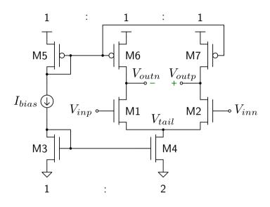
$$\left\{egin{array}{l} V_{ind} \doteq V_{inp} - V_{inn} \ & V_{inc} \doteq rac{V_{inp} + V_{inn}}{2} \ & V_{outd} \doteq V_{outp} - V_{outn} \ & V_{outc} \doteq rac{V_{outp} + V_{outn}}{2} \end{array}
