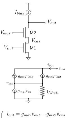
$$\begin{cases} i_{out} = g_{md2}v_{out} - g_{ms2}v_{cas} \\ g_{md1}v_{cas} = i_{out} - g_{mg1}v_{in} \end{cases}$$
