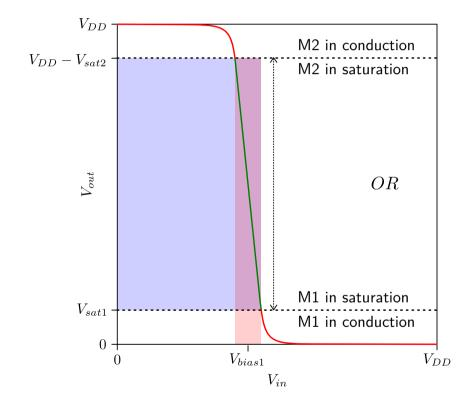
$$OR = V_{DD} - V_{sat1} - V_{sat2}$$
