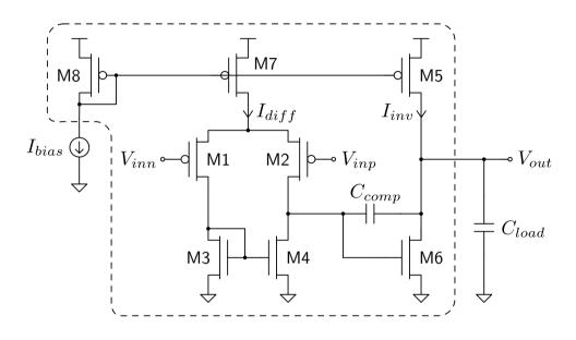
$$GBW = \frac{g_{mg1,2}}{2\pi C_{comp}} = \frac{1}{2\pi C_{comp}} \sqrt{\frac{\beta_P}{n} \left(\frac{W}{L}\right)_{diff}} I_{diff}$$
