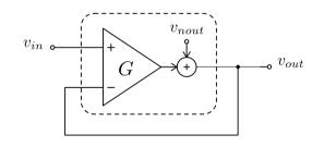
$$v_{out} = v_{nout} + G(v_{in} - v_{out})$$
