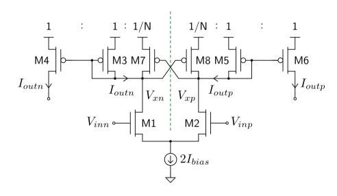
$$i_{outn} = g_{mg1} \frac{v_{ind}}{2} \frac{g_{mg3}}{g_{mg3} - g_{mg7}}$$
