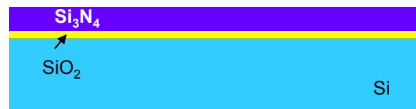
Deposition of trench filling oxide (No thermal growth!)
