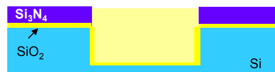
Oxide CMP polish step with stop on nitride
