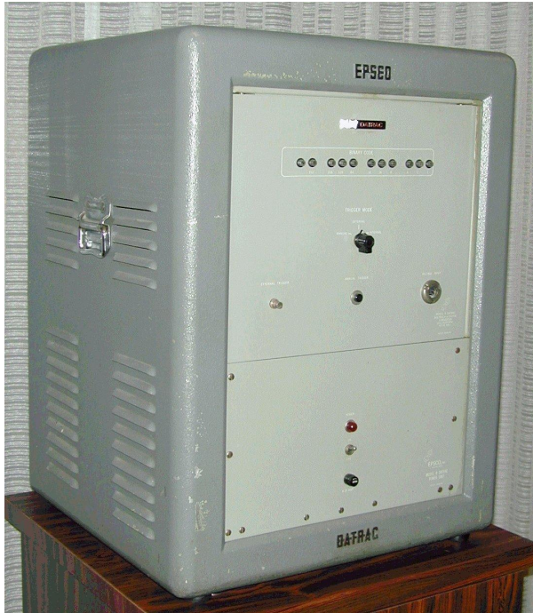
EPSCO DATRAC, B.M. Gordon, 1953 11-bit 50KSps 500W SAR ADC 0.5m x 0.4m x 0.65m, 70Kg Vacuum tube technology
