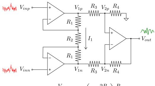
$$G_d \doteq \frac{V_{out}}{V_{inp} - V_{inn}} = \left(1 + \frac{2R_1}{R_2}\right) \frac{R_4}{R_3}$$
