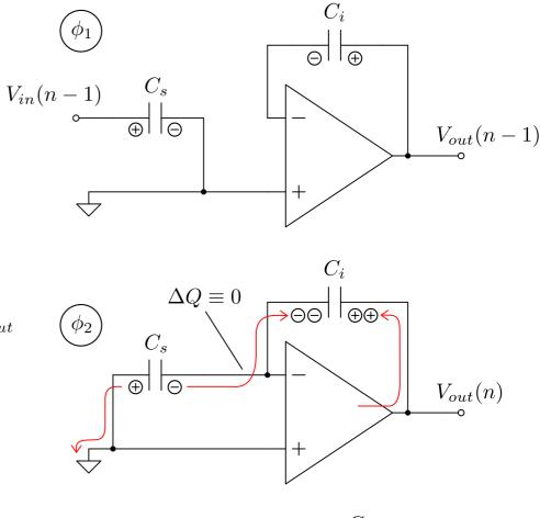
$$V_{out}(n) = V_{out}(n-1) + \frac{C_s}{C_i}V_{in}(n-1)$$
