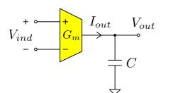
$$G_m \doteq \frac{I_{out}}{V_{ind}} = 2\sqrt{\frac{2\beta I_{tun}}{n}}$$
