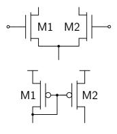
multiplicity (**M**) design for a common channel aspect ratio (W/L)
