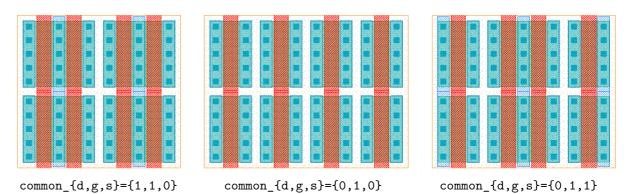
e.g. CNM25 NMOSFET parameterized cell (PCell)
