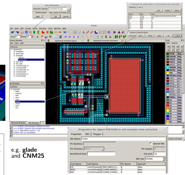
opamp\_par.sub .SUBCKT opamp vinn vinp vout vdd vss ibias MM0 vdd ibias vdd vdd cnm25modp w=1.2e-05 l=6e-06 as=... MM1 vdd ibias vout vdd cnm25modp w=1.2e-05 l=6e-06 as=... Cc0 vinter vout cnm25cpoly w=6.42928e-05 l=0.000156207 MM8 vout ibias vdd vdd cnm25modp w=1.2e-05 l=6e-06 as=... ... CP1 vinter vss C=3.8582e-13 CP2 vout ibias C=3.33692e-15 CP3 vinp vss C=1.85938e-15 CP4 vout vcomm C=2.0918e-15 ...
