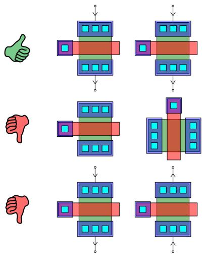
Anisotropic materials (e.g. wafer crystal lattice orientation)
