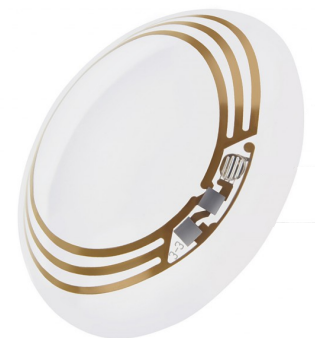
Wireless contact lens for health monitoring
