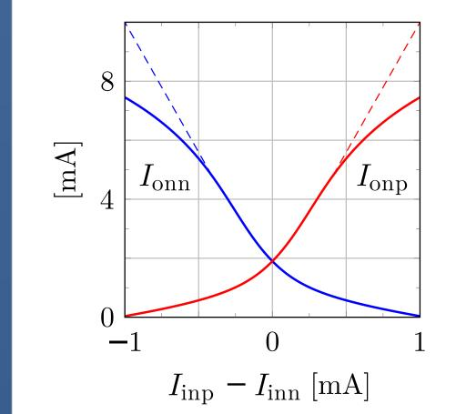
As shown, the number of transistor groups is minimized and minimum device lengths can be used. In this particular case, optimization finds the best performance for A=4, B=3 and C=1. The Class-AB behavior is demonstrated for the NMOS outputs.
