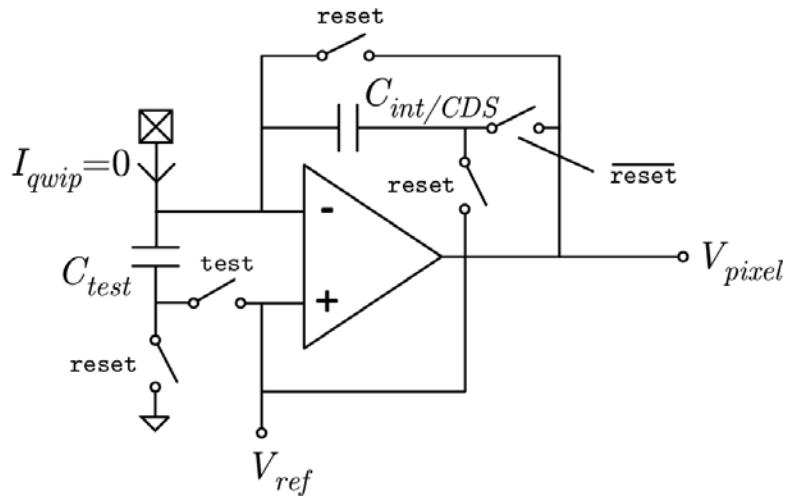
$$V_{pixel} = \left( 1 - \frac{C_{test}}{C_{int/CDS}} \right) V_{refi}$$
