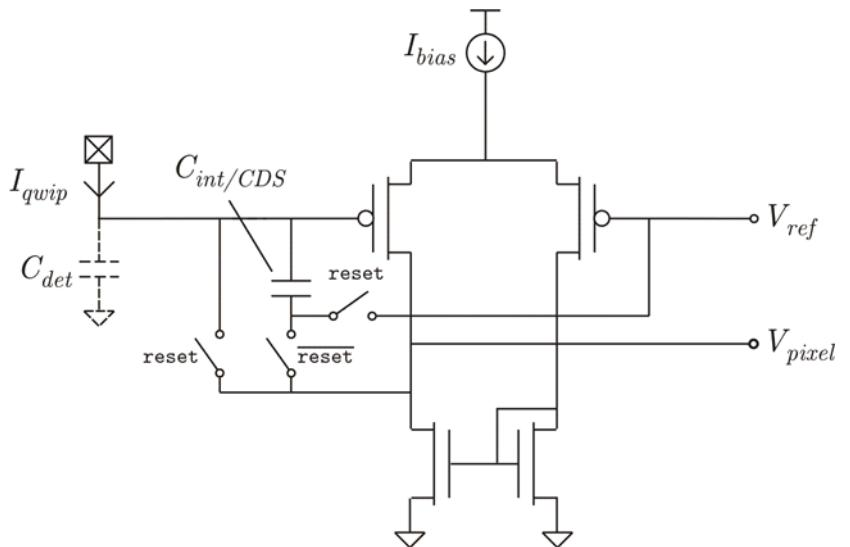
Open loop gain has to be high enough to lower the input impedance and assure a high current injection efficiency.
