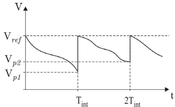
$$V_{pixel} \simeq V_{ref} - \frac{T_{int}}{C_{int}} \cdot I_{qwp}$$
