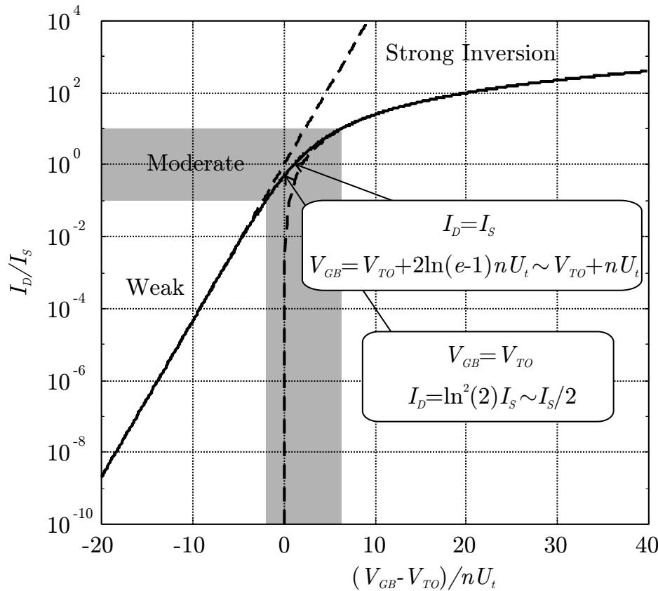
$$I_D = I_S e^{\frac{V_{GB}-V_{TO}}{nU_t}} e^{-\frac{V_{SB}}{U_t}} \quad IC = \frac{I_D}{I_S} \ll 1$$
