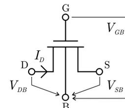
$$I_D = I_S e^{\frac{V_{GB}-V_{TO}}{nU_t}} e^{-\frac{V_{SB}}{U_t}} \quad I_S = 2n\beta U_t^2$$
